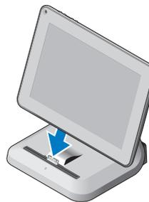
Align the computer with the docking station connector and press down until it clicks into place.
